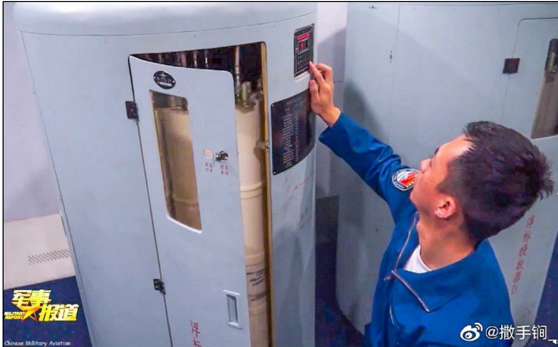
Figure 6: Sonobuoy Cabinet on KQ-200 69
